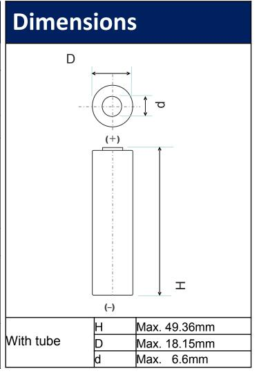
When designing a pack, refer to the cell's mechanical drawing for precise dimensions.
