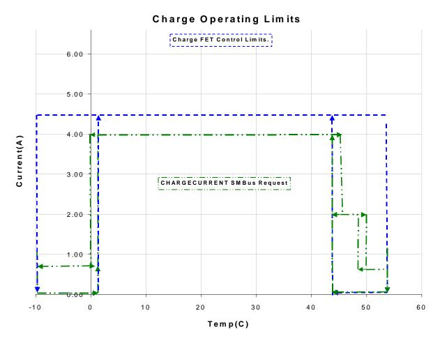
NOTE: If not charging & temperature > 45C then the battery enters Charge-Inhibit where ChargeCurrent() = 0 until temperature < 44C.
