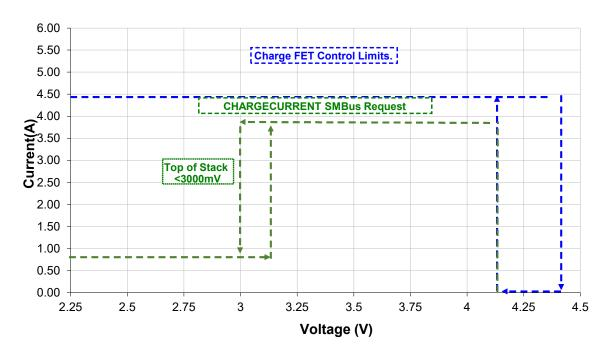
NOTE: The charging current requested from 3.0 to 4.2 V is defined by the temperature of the pack as shown in the preceding charge operating limits graph in this section. A 4.0A charge current is shown in this graph to represent the current defined by said graph.
