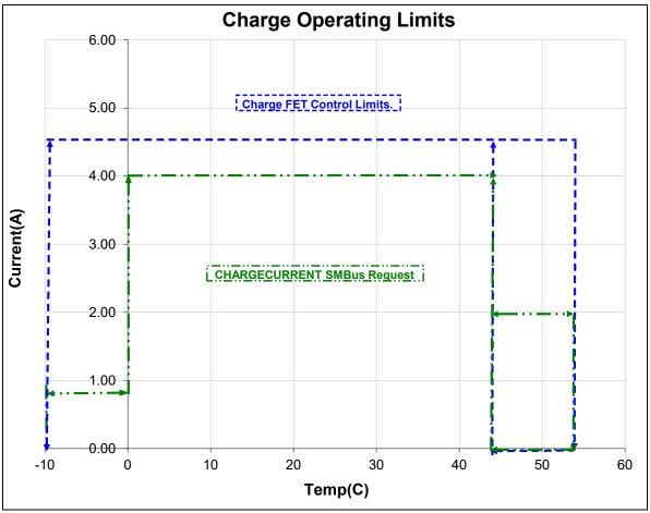
NOTE: If not charging & temperature > 45C then the battery enters Charge-Inhibit where ChargingCurrent() = 0 until temperature  $\leq$  44C.
