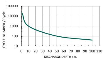
Charging Condition : CV(3.4V,  $160\Omega$ , 48H) Discharging Condition : CR( $30k\Omega$ , 2.5V Cut-off)
