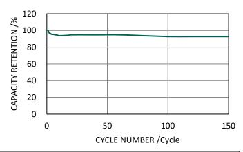
Charging Condition : CV(2.3V, 200 $\Omega$ , 7H, 20°C) Discharging Condition : CR(10k $\Omega$ , 1.0V Cut-off, 20°C)
