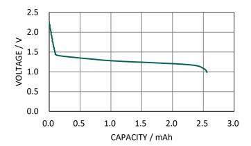
Charging Condition : CV(2.3V, 300 $\Omega$ , 16H, 20°C) Discharging Condition : CR(30k $\Omega$ , 1.0V Cut-off, 20°C)
