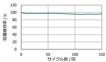
Charging Condition : CV(2.3V, 750 $\Omega$ , 8H, 20°C) Discharging Condition : CR(10k $\Omega$ , 1.0V Cut-off, 20°C)
