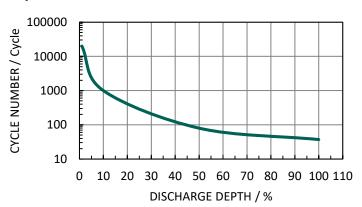
Charging Condition : CV(3.4V, 560  $\!\Omega$ , 48H) Discharging Condition : CR(100k  $\!\Omega$ , 2.5V Cut-off)
